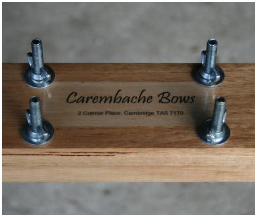
Figure 1 - Laminating/Straightening Jig - Detail
