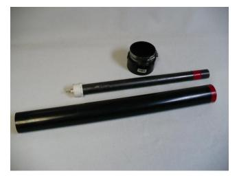
The SCA published a method for testing fencing armour in its 2006 website at SCA.org. It uses a Meyer standard 1/8" drop pin on a heavy tube, and its drop height was designed to exert 1.5 Joules of force onto the material being tested -- a much more scientifically accurate system than banging the armour into the dirt with a broken foil.
